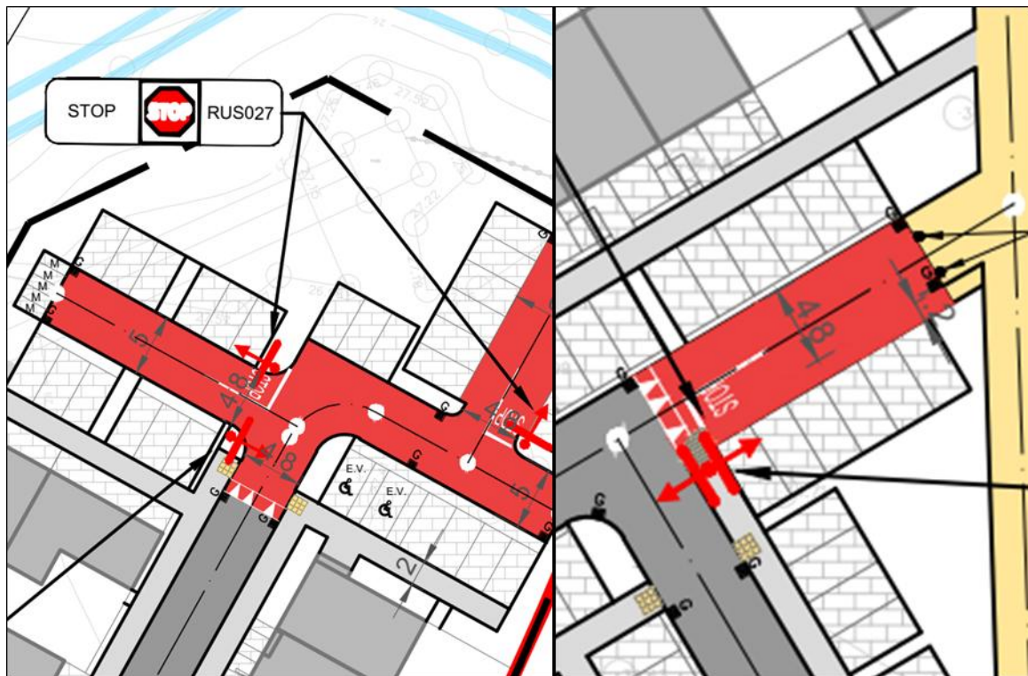
Figure 2.1 Parking Aisles Designated as 20 km/h Shared Space
